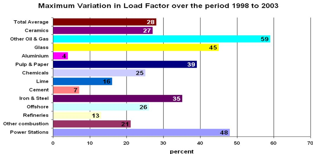
Figure 1: Production variations of *existing* manufacturing plants of various sectors in the six year period 1998-2003 in the UK reported by Entec-NERA. The average score was 28%.
